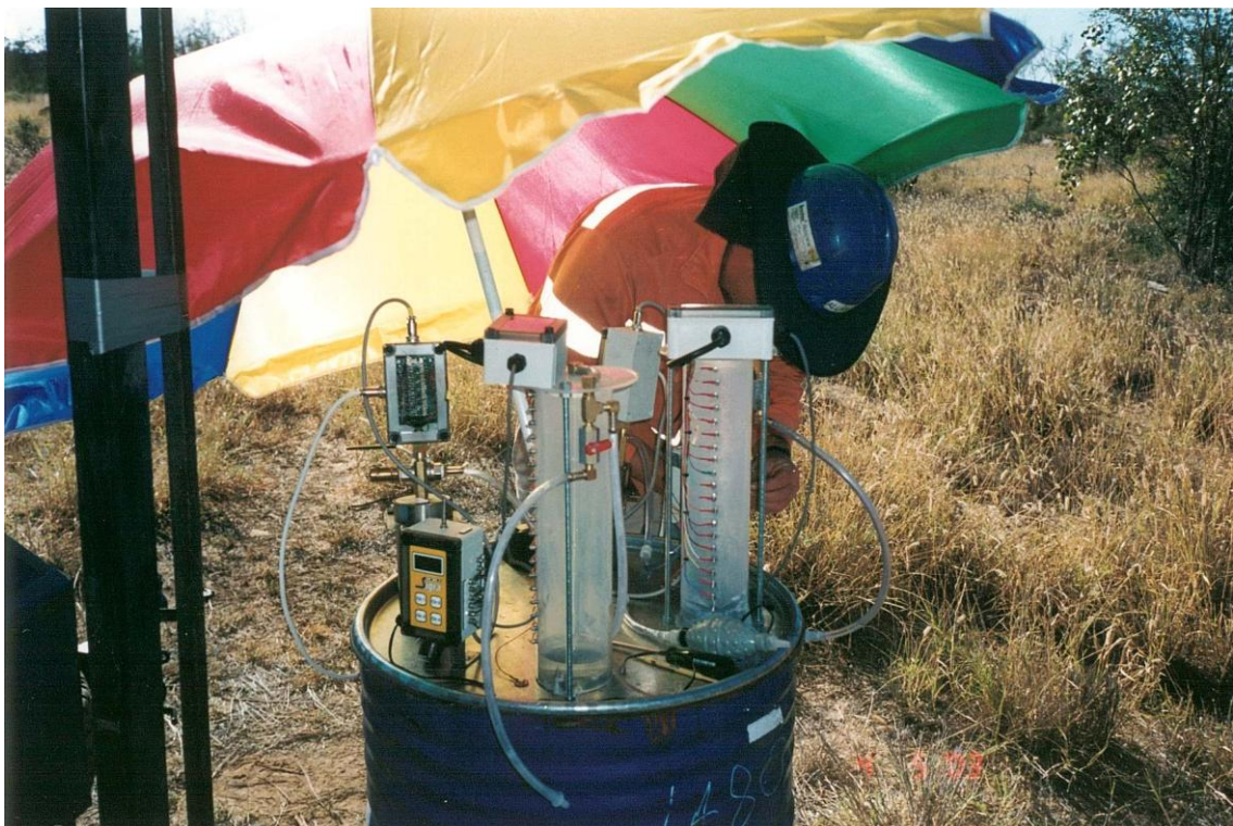
Set-up for testing coal shrinkage with desorption
