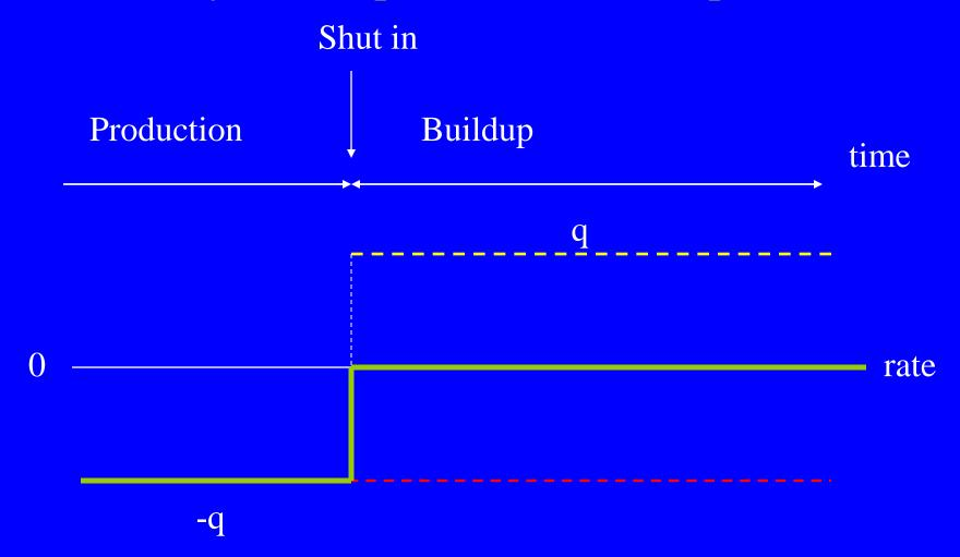
For production / buildup test, a production rate q occurs for time t and is followed by a shut-in / buildup period for time delta t.
