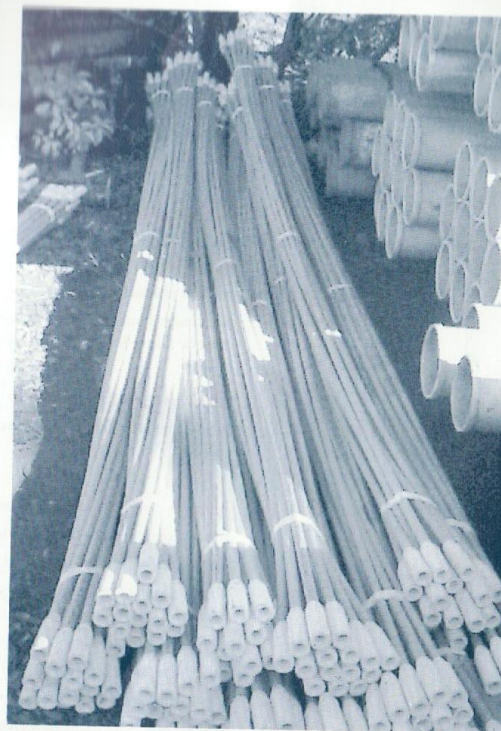
Surveying Conduit for pushing Camera up the hole to be surveyed
