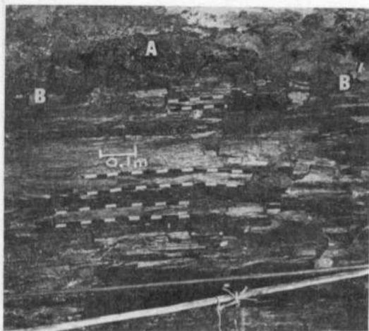
Fig. 10 - View of uppermost 1 m of coal in 53 west-level, showing numerous rod structures. The traces of some rods are marked. A is the stone roof and B-B' is the coal/stone parting.
