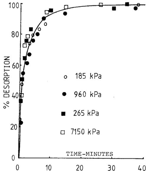
Fig.1 - Desorption of sample E, Bulli Seam, West Cliff Colliery (-53 um) at 30°C for a range of equilibrium methane adsorption pressures.
