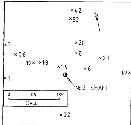
Fig.2. -  $\text{CO}_2$  concentration in Bulli Seam gas at West Cliff Colliery, N.S.W. e.g. x 1 = 1%  $\text{CO}_2$
