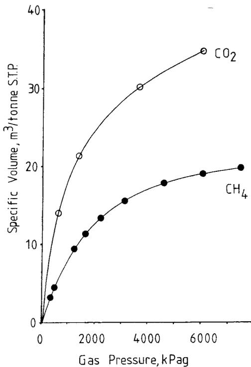
Fig. 3. Equilibrium Desorption Isotherms for Bulli Seam coal, West Cliff Colliery, 30°C, 0% moisture. (Hayes, 1982).
