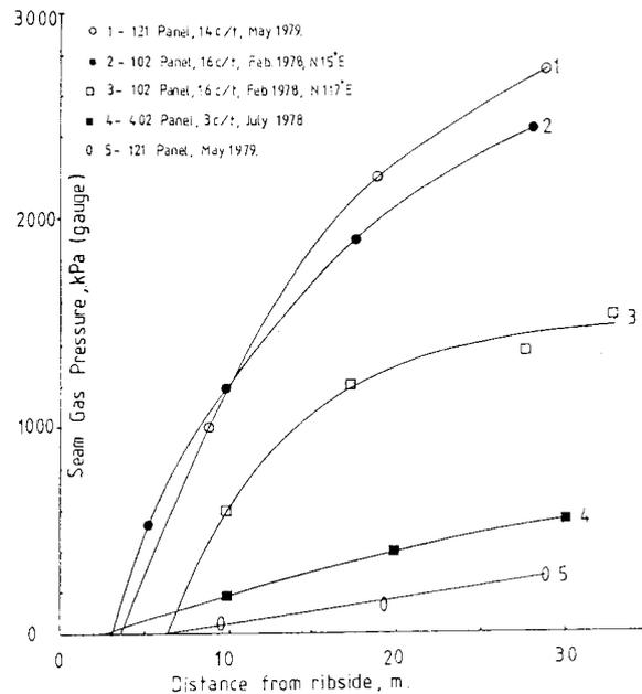
Fig. 4. Variation of seam gas pressure with distance into solid coal, West Cliff Colliery, Appin. The depth of the crushed zone can be calculated where the pressure is zero, and varies from 2.5 to 6.5 m.
