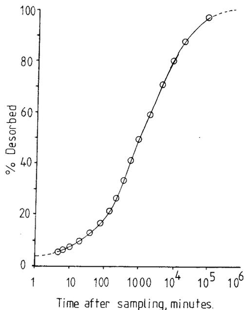
Fig. 6. Desorption of a face sample from West Cliff Colliery:  $-73 \pm 3$  mm, original gas content  $10.8 \text{ cm}^3/\text{g}$ ; 0.9% moisture; seam gas 99%  $\text{CH}_4$ .
