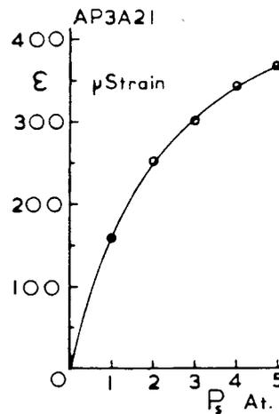
Fig. 5. Circumferential strain detected in typical core as sheath pressure ( $P_s$ ) changes.
