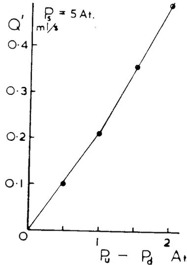
Fig. 3. Normalised air flow rate ( $Q' = Q/P_m$ ) versus pressure drop for upstream pressure great enough to produce partial "lift-off" of rubber sheath.
