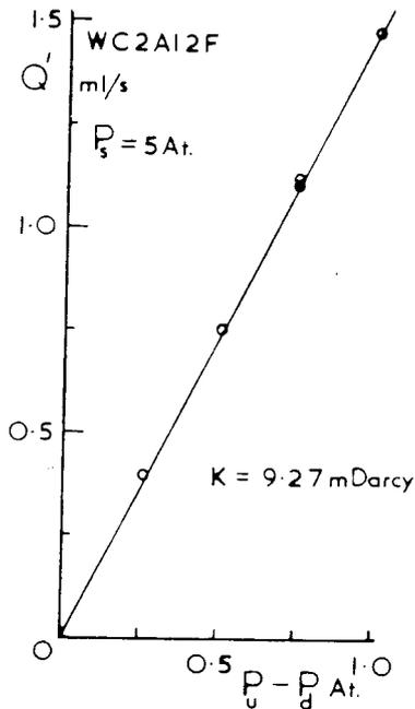
Fig. 2. Normalised air flow rate ( $Q'$ ) versus pressure drop for typical core,  $P_s$  = sheath pressure.
