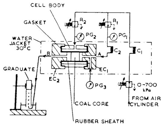
Fig. 1. Laboratory Permeameter - See text for detailed description
