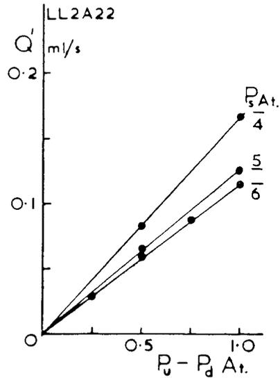
Fig. 4. Effect of radial sheath pressure ( $P_s$ ) on flow rate  $Q'$  at series of driving pressures.
